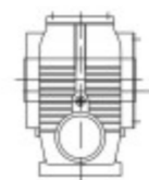
RCSA..D.. 空心軸安裝斜齒輪--蝸輪蝸杆齒輪減速電機 Helical – worm gearmotor with hollow shaft.
