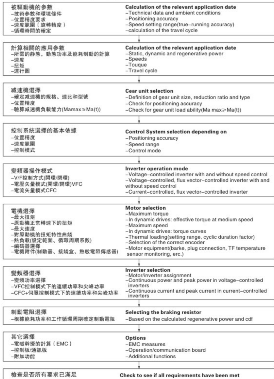
圖：選型應用流程圖 Figure:Project planning process
